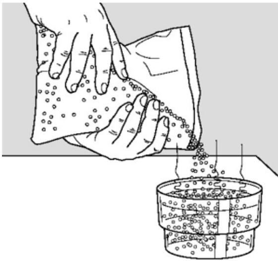
1. Pour ALLFIT in a Suspan (Art.no. 35240), a water heater or a bowl of hot water at 65°C (149°F) or more.
