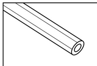
Tube (polycarbonate) into which a braided elastic or extension spring is introduced, provides a spatial suspension point for the finger.
