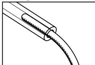
Synthetic thread used to prevent kinks from arising when the ORFITUBE is shaped.
