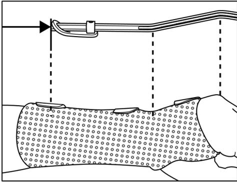
11. For a few seconds, heat the underneath of the ORFITUBE ADJUSTER as well as the attachment location on the orthosis with a heat gun (be careful for overheating).
