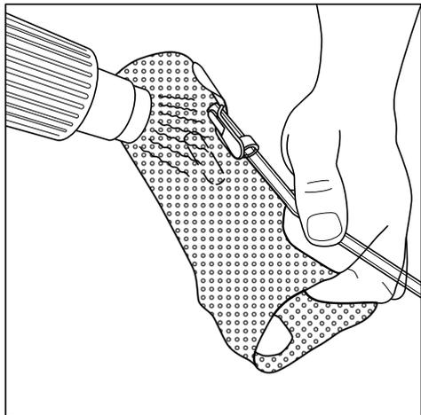
12. Firmly press the ADJUSTER onto the orthosis in the desired position and allow it to cool down completely.
