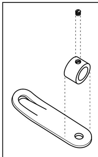
Adjusting ring (Polyacetal): Holds and allows alterations of the ORFITUBE.
