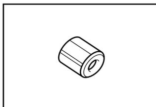
Metal cap (nickel-coated brass) with rounded edges, to reduce friction of the elastic.
