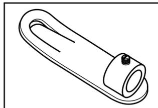
Adjusting screw (stainless steel): Secures the position of the ORFITUBE in the adjusting ring.
