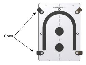
Form the mask. Make sure the UON frame is positioned over the indexing pins on the base plate. Then close the swivel locks by turning them over the frame. See picture below.
