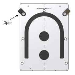
Form the mask. Lock the mask down using the DUON push pins. Then close the swivel locks by turning them over the frame. See picture below.
