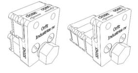
The blocks snap onto the AIO FIX: no tooling is required.
