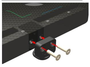
Mount the Loxon blocks to the side of the base plate using the plastic countersunk M5 x 20 screws and a screwdriver.
