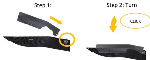
Removing a lateral profile from the base plate:
