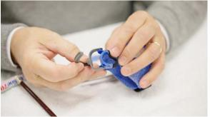
14. Check if the Isoforce unit moves easily forward and back with the pegs securely embedded in the holes.
